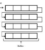
Fig4. FIFO Architecture
