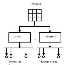
Fig2.CBHR Concept in NoC Architecture
